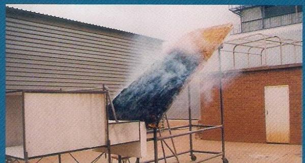
*Spread of flame test: Burner extinguished*
